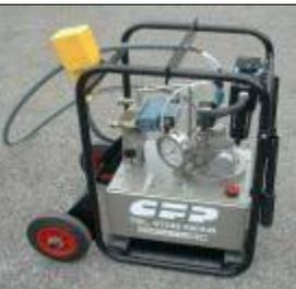
700 bar air driven power pack for use underground with pendant mounted controls for ram directional control and motor run. Built for Hi Torque Ltd.
