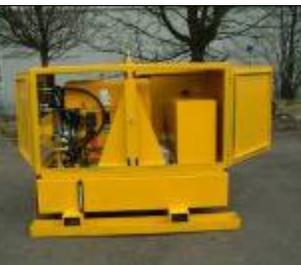
Diesel driven power packs for Forker Plant. Required to deliver dual volumes to drive 'slip pumps'. Included access doors and canopy.
