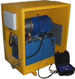
Build and test of ten hydraulic power units; each operating two rams, for waste reclamation company. Included cabinet, pump, electric motor, res tank, filters, pressure regulation, control valves, internal piping, instrumentation and spillage trays.
