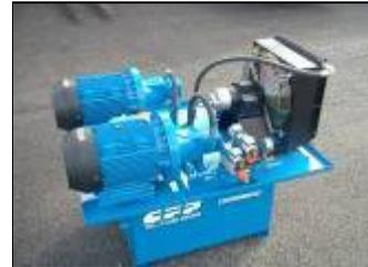
Twin pump power pack used to drive an engine block 24hours per day, 7 days per week for Jaguar Cars. Built for T.Q.C. Ltd, Notts.
