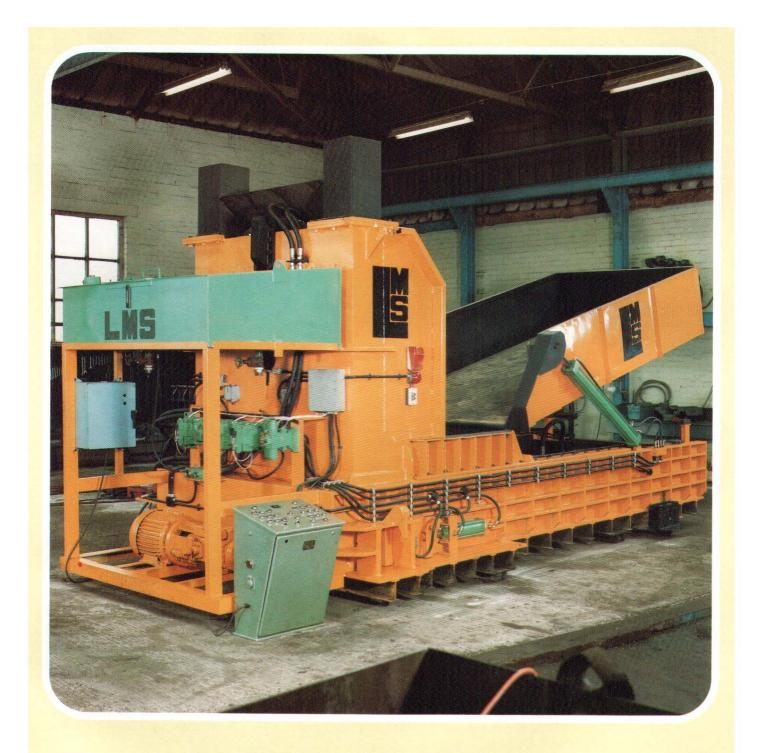
This has proved to be an ideal machine for small to medium sized scrap yards where there is a need for an inexpensive and simple baler capable of handling all types of ferrous and non-ferrous bulky scrap. Materials such as Car Shells, Cookers, Fridges, Washing Machines, Factory Cuttings, Aluminium etc. are ideal for this machine.
