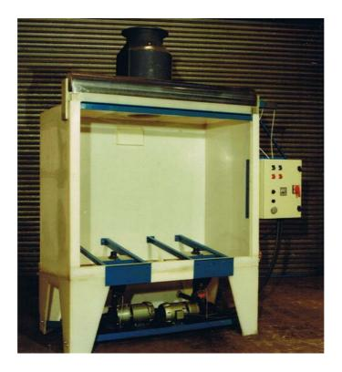
The Challenger Drumtech Internal Acid De-rusting Machine is designed to de-rust the inside of open and closed top 205-litre steel drums.
